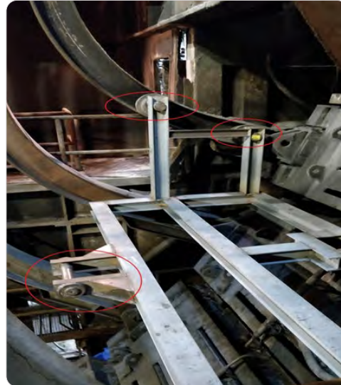
Picture 6: Wheels and lifting lug details during previous test. Picture courtesy of Acerinox Europa.
